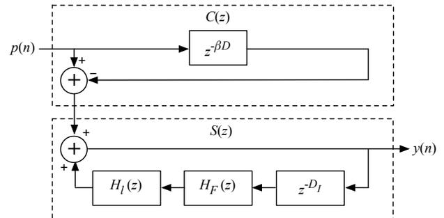
**Figure 1: Source-filter model for plucked-guitar synthesis.**  $C(z)$  simulates the effect of the player’s plucking position.  $S(z)$  models the string’s pitch and decay characteristics.
