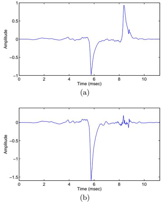
**Figure 2: Plucking point compensation for a residual signal obtained from plucking a guitar string 8.4 cm from the bridge (open E,  $f_0 = 331$  Hz). (a) Without and (b) with equalization**
