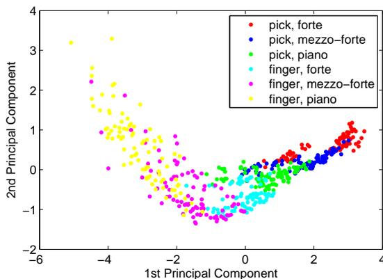
Figure 4: Projection of guitar excitation signals along the first two principal axes.
