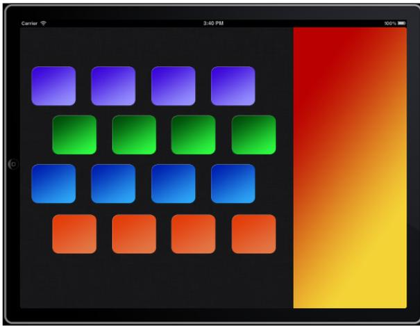
**Figure 7: Tabletop guitar interface for the components based excitation synthesis. The articulation is applied in the gradient rectangle, while the colored squares allow the performer to key in specific pitches.**
