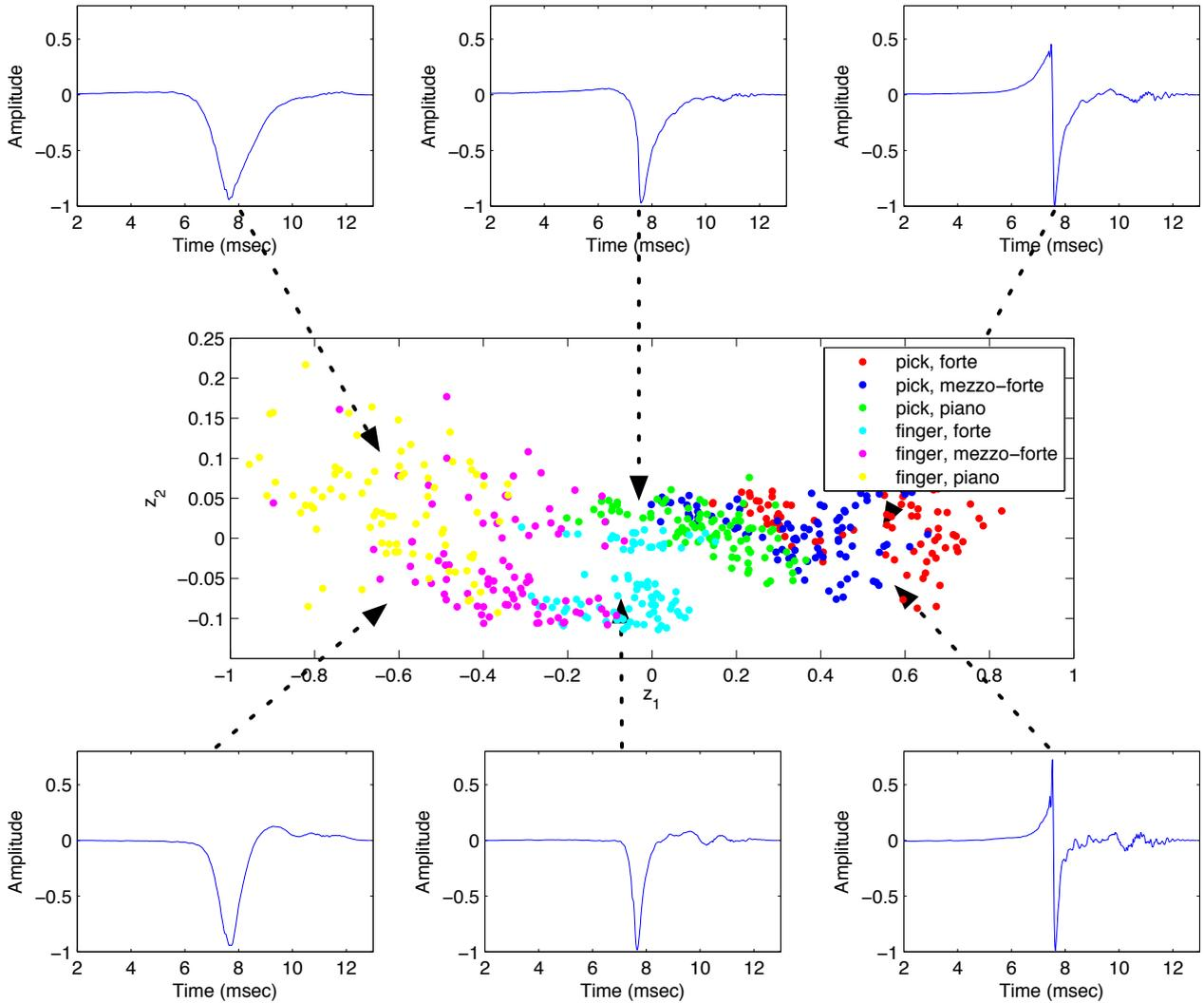
**Figure 6: Projection of the guitar data into the reduced dimensionality space defined by the ANN (center). Example excitation pulses resulting from sampling this space are also shown.**
